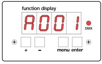
If the led is off, the projector is not receiving signal. Check the cabling and the functioning of the controller.
