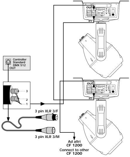
Ensure that all data conductors are isolated from one another and the metal housing of the connector
