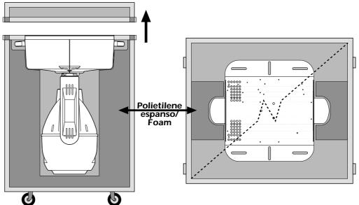
B) Fixing the base to a rigid support, with padding surrounding the articulated head.
