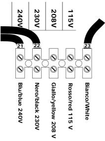
Incorrect voltage selection will detrimentally affect the operation of the projector. Under no circumstances should cable 23 be moved.
